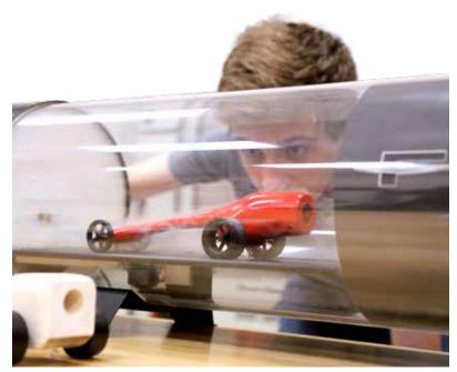
The presence of eddies indicates that features of your car body are causing aerodynamic drag. Streamlining such features can improve the efficiency of the car's shape and help it cheat the wind as it moves down the track. The bottom line: more speed!
