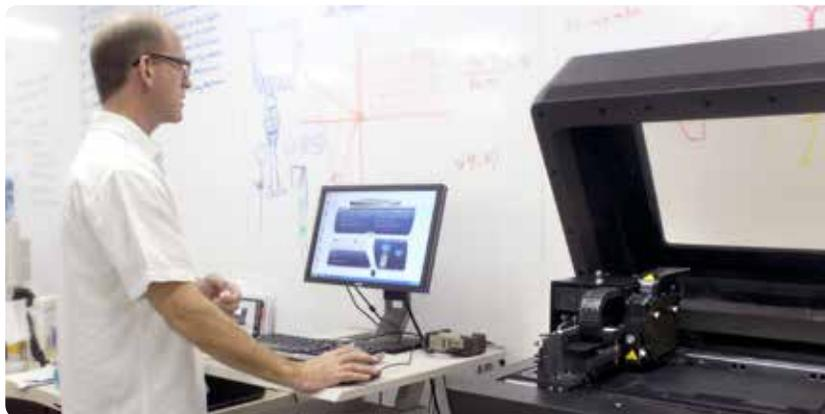
1. First, the desired object is created as a 3-D model within a CAD software program and sent to the 3-D printer. After the printer is warmed up, the printing begins.
